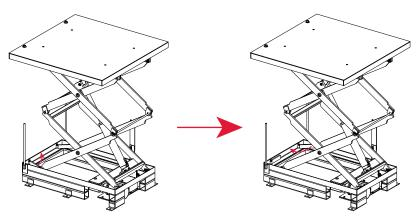
5. Press and hold the **DOWN** button to lower the lift table to ground or lowest height position then release the button.
