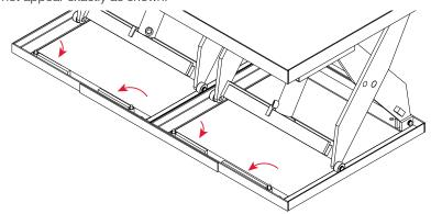
Press and hold the **DOWN** button to lower the lift table to ground or lowest height position then release the button.
