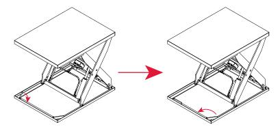
Press and hold the **DOWN** button to lower the lift table to ground or lowest height position then release the button.
