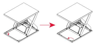
5. Press and hold the **DOWN** button to lower the lift table to ground or lowest height position then release the button.
