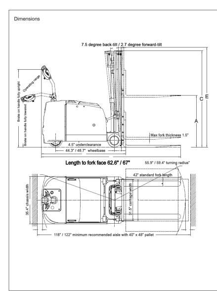
Aisle Guide BGL-30 Right Angle Stacking
