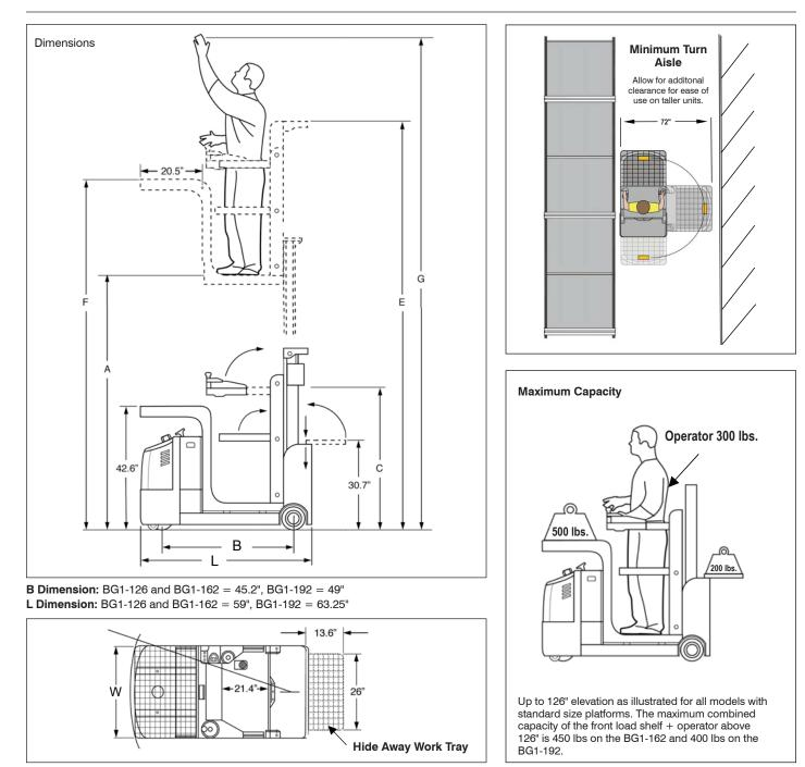
W Dimension: BG1-126 and BG1-162 = 31.5", BG1-192 = 34" Turning Radius: BG1-126 and BG1-162 = 52.5", BG1-192 = 56"
