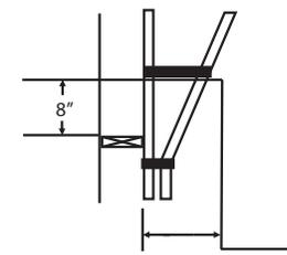
Please provide measurement (in inches) from the wall to the edge of the door track at approximately 8" above the header.
