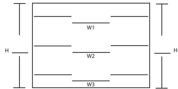
Please provide the measurements of the height and width (in inches) at the top, center, and bottom of the opening.
