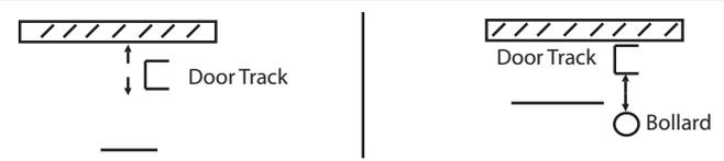
Please provide the projection from the wall to the front of the existing door tracks. If bollards are present, please provide measurement between the door track and the bollard.
