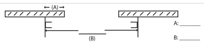
If the mount style is Inside Stand-Off, please provide the measurement from the jamb to the inside of the track (A) and the width of the existing door guide tracks (B).
